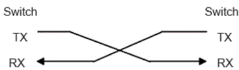
Figure 7-1 Optical Cable Connections
